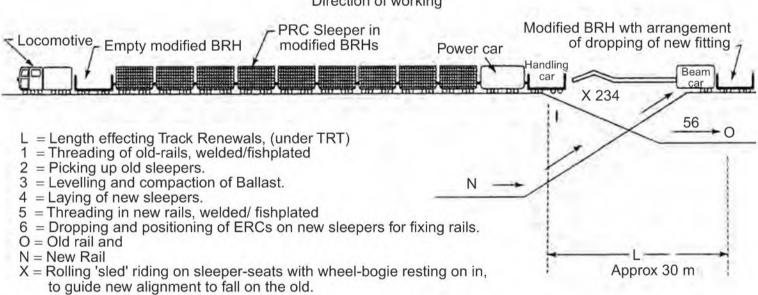
Fig. 15.8 Composition of ART with modified BRHs and track renewal mechanism
