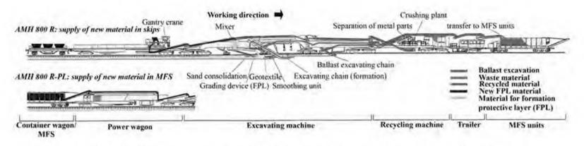
Fig. 12.18 Formation rehabilitation machine (See also Color Plate 9)
