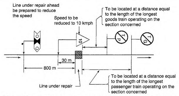
Fig. 11.7 Works of long duration providing protection by reduced speed outside station limits
