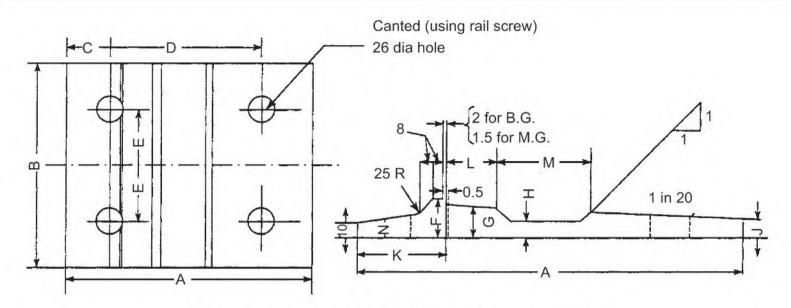
Fig. 5.6 Single rail MS bearing plate (canted)
