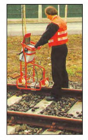
Fig. 10.15 The rail scan equipment
