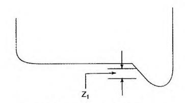
Fig. 22.26 Safety depth of flange
