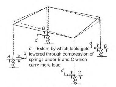
Fig. 22.24 Table on ground level conditions with legs resting on springs instead of directly on ground
