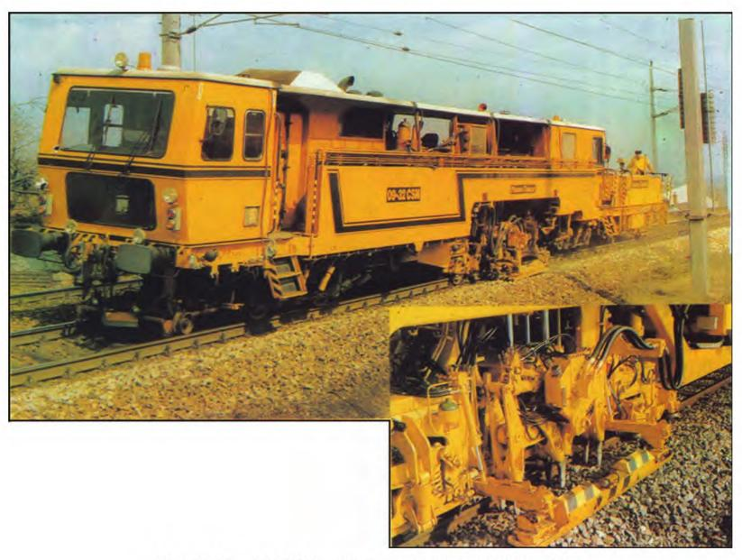
Fig. 12.13 09-CSM continuous action tamping machine
