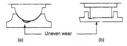
Fig. 22.45 (a) Uneven wear in hemispherical pivot (b) Uneven wear in flat pivot
