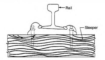
Fig. 5.8 Anti-creep nearing plate
