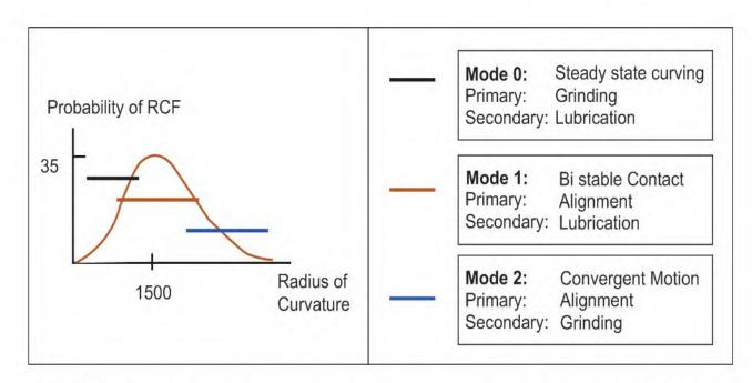
**Fig. 2.5** RCF initiation modes as a function of curvature and recommended track based remediation. Overl apping influence rather than distinct boundaries exist between modes
