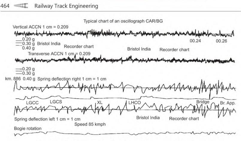
Fig. 17.4 A copy of sample chart obtained from an oscillograph car
