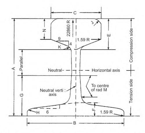
Fig. 2.3(b) British Standard F.F. rail section—key to table of dimensions
