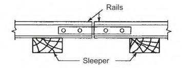
Fig. 3.5 (b) Suspended joint
