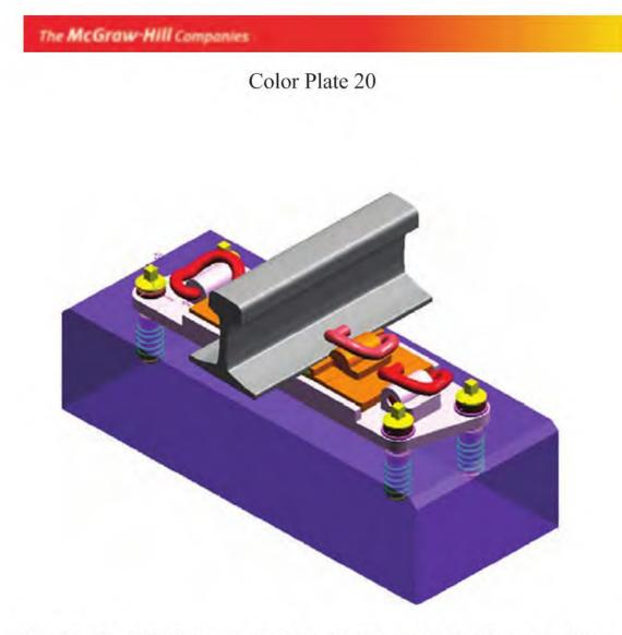
Fig. 21.12 Plinth type ballastless track assemblies for main lines
