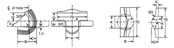
Fig. 5.18 Spring steel loose jaws
