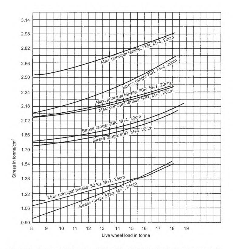
Graph I Stresses in bolt holes of 52 kg 90R, and 75 R rails (for broad gauge track)
