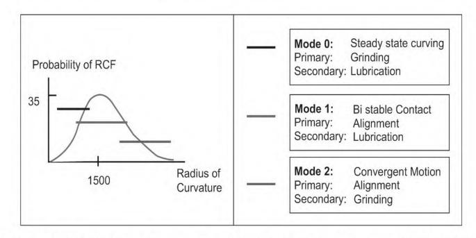
**Fig. 2.5** RCF initiation modes as a function of curvature and recommended track based remediation. Overlapping influence rather than distinct boundaries exist between modes (See also Color Plate 1)
