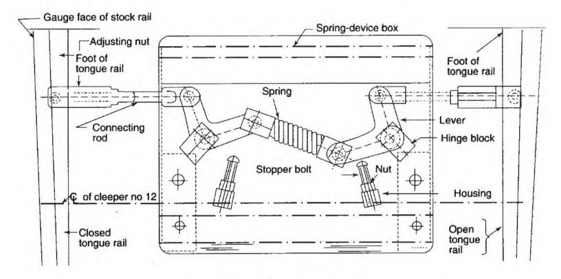
Fig. 7.31 Spring operated device
