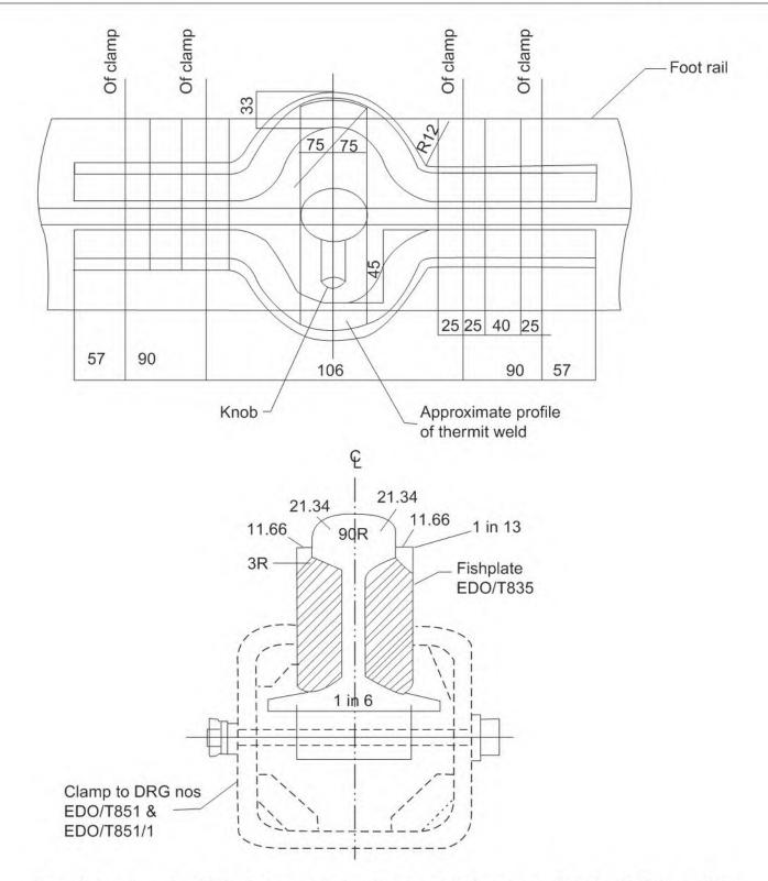
**Fig. 3.7** Joggled fishplates and clamps for rail fractures BG for BS No. 90R
