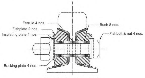
Fig. 3.8 Insulated rail join
