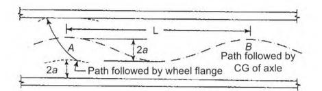
Fig. 22.21 Sinusoidal motion of centre of gravity of coned wheel set
