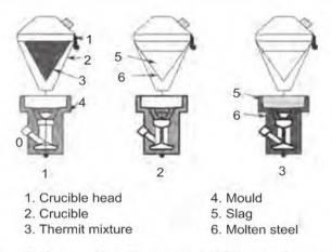
Fig 9.2 Schematic diagram of Thermic method
