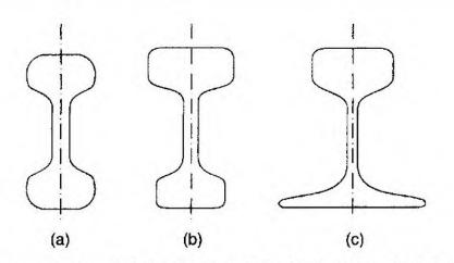
Fig. 2.1 Type of rails: (a) double-headed; (b) bull-headed; (c) flat-footed
