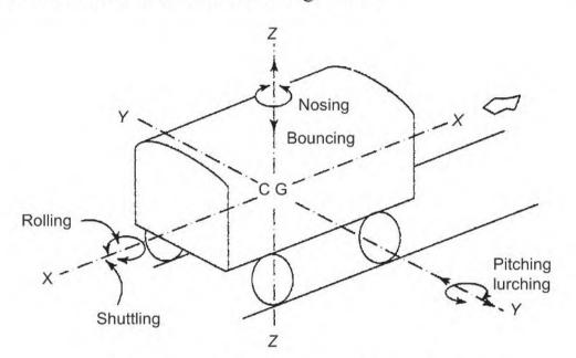
Fig. 22.18 The six modes of oscillation
