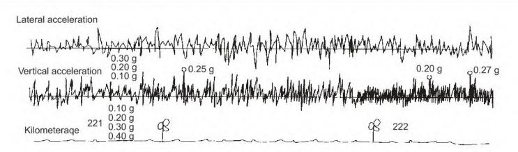
Fig. 17.5 Sample chart of portable accelerometer
