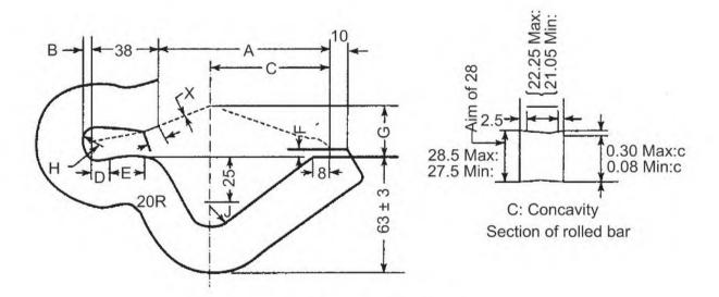
Fig. 5.37 Rail anchors
