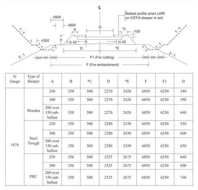
1. The minimum clean stone ballst cushion below the bottom of sleeper, i.e., A = 250 mm.
