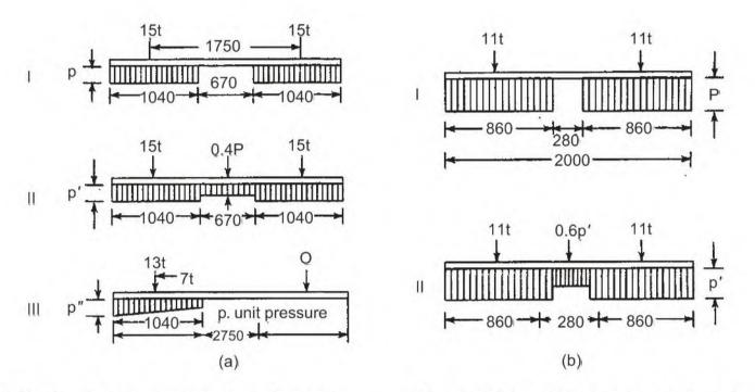
Fig. 4.19(a) BG sleeper-loading diagram
