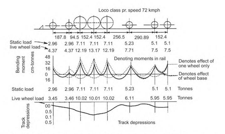
**Fig. 19.1** Rail bending moments and depression curves for 4-6-2 locomotive
