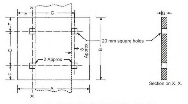
Fig. 5.5 Single rail mild steel bearing plate-flat
