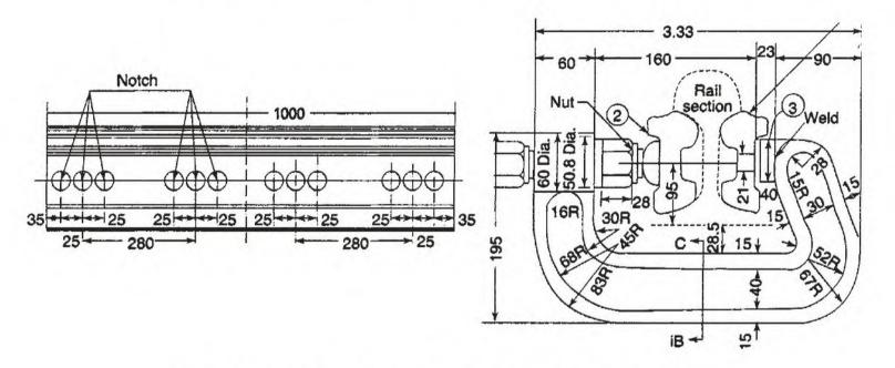
Fig 10.11 1000 mm long special fishplate for clamped joints
