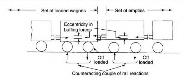
**Fig. 22.46** Effect of vertical eccentricity in buffing forces at junction of a set of empties and a set of loaded wagons
