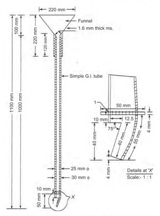
Fig. 14.18 Packing tube for measured tube packing of ST sleepers BG
