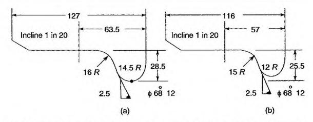
Fig. 22.28 Profile of a new wheel with standard flange (a) BG wheel (b) MG wheel, (all dimensions in mm)
