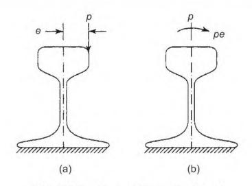
Fig. 19.3 Eccentric vertical load
