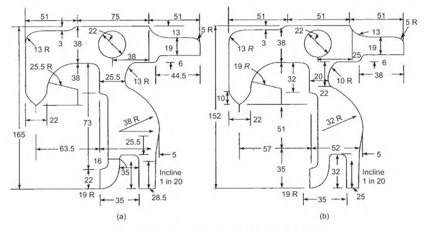
Fig. 22.29 Type defect gauge (a) BG (b) MG
