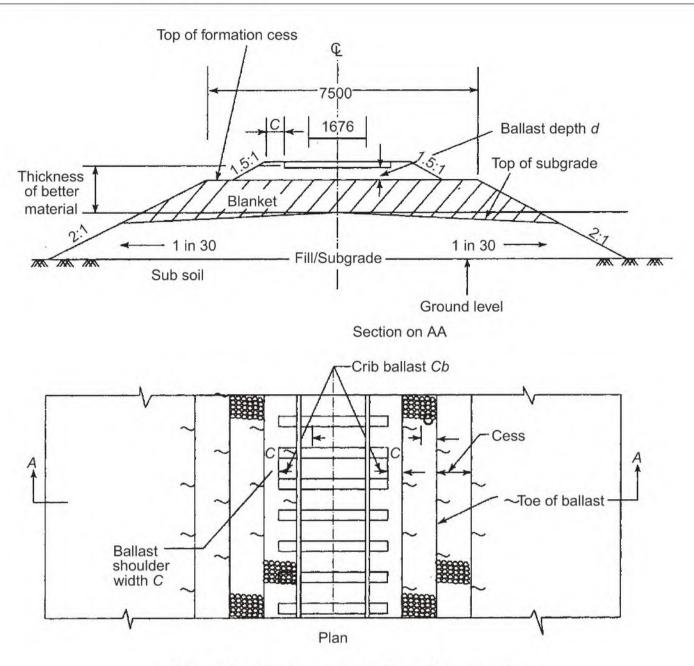
Fig. 8.1 Cross-section of a railway track
