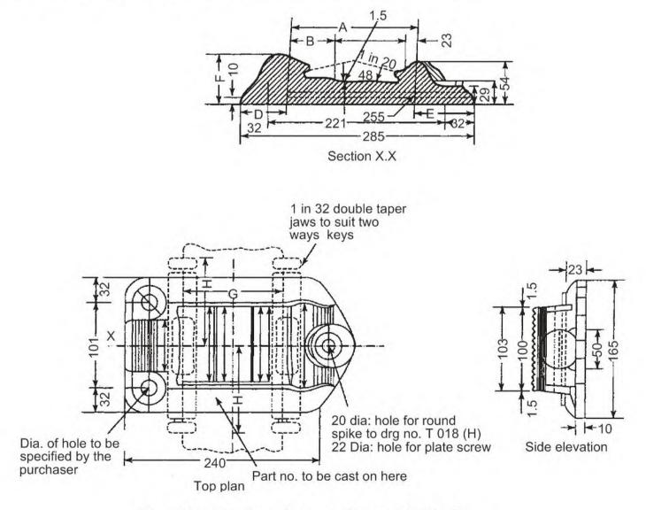
Fig. 5.9 Bearing plates, anti-creep CI (MG)
