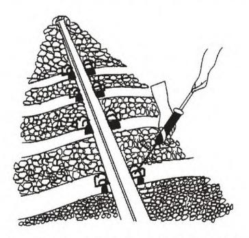
Fig. 20.2 Injecting epoxy resin into 'Pandrol' shoulders
