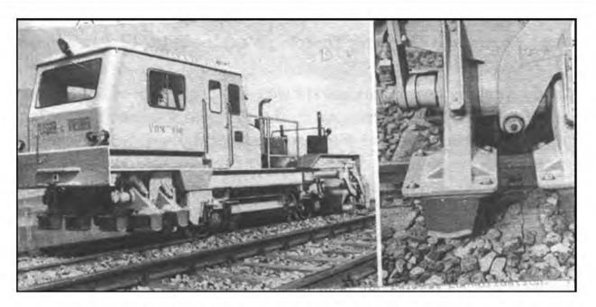
Fig. 12.10 Sleeper crib and shoulder consolidating machine
