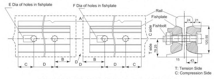
Fig. 3.3 (e) Fishplate for 60 kg rails (refer to Table 3.5)
