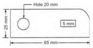
Fig. 15.3 Sketch showing a liner
