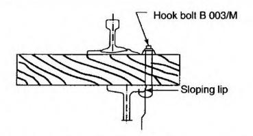
Fig. 5.36 Method of fastening wooden sleepers on joist spans
