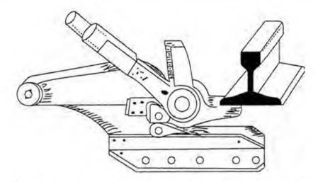
Fig. 14.7 Non-infringing type of mechanical jack
