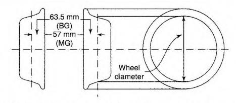
Fig. 22.17 Measurement of wheel diameters on the same axle
