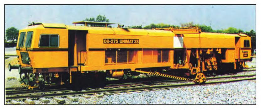
Fig. 12.11 (b) Unimat 08-275 3S switches and crossing tamping machine
