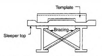
Fig. 21.1 (d) Checking of notches surfaces to be in one plane
