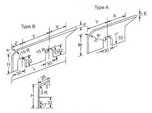
Fig. 3.4 Tapered shim
