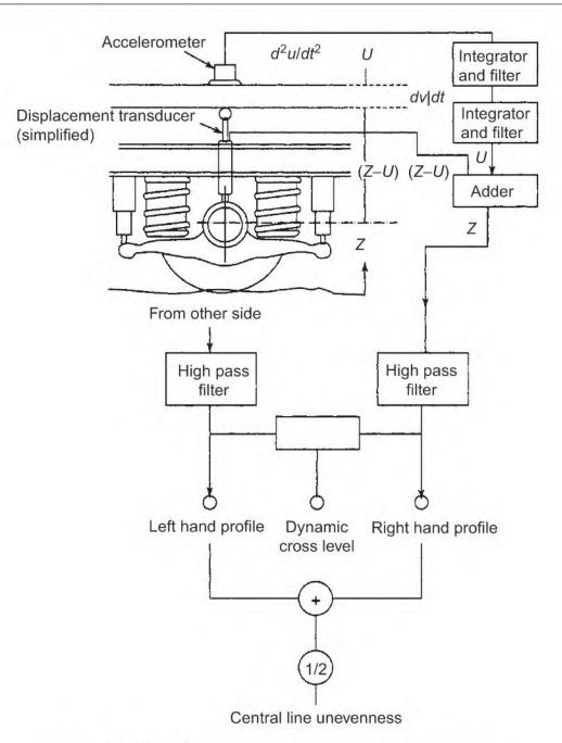
Fig. 17.14 Vertical profile system (schematic)
