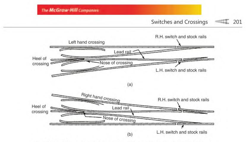
Fig. 7.13 Turnouts-crossings and switches: (a) left hand; (b) right hand
