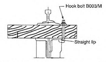
Fig. 5.35 Method of fastening wooden sleepers on plate girder spans
