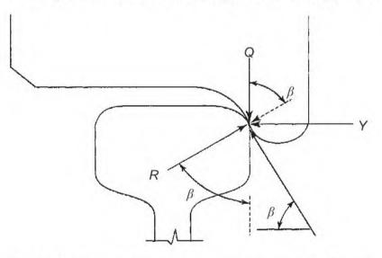
**Fig. 22.13** Forces at rail-wheel contact at moment of incipient derailment with positive angularity of axle
