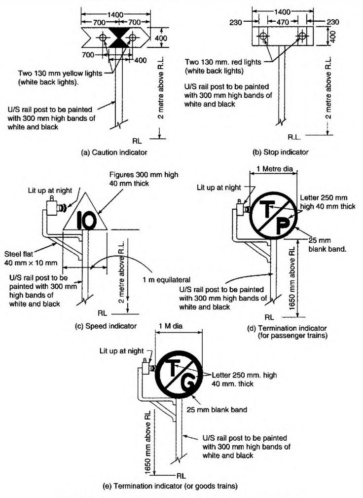
Fig. 11.3 Engineering indicators for temporary restrictions
