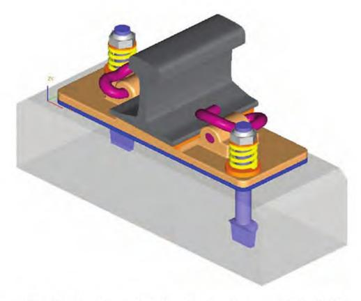
Fig. 21.11 Logwell ballastless track assembly (LM-1)
