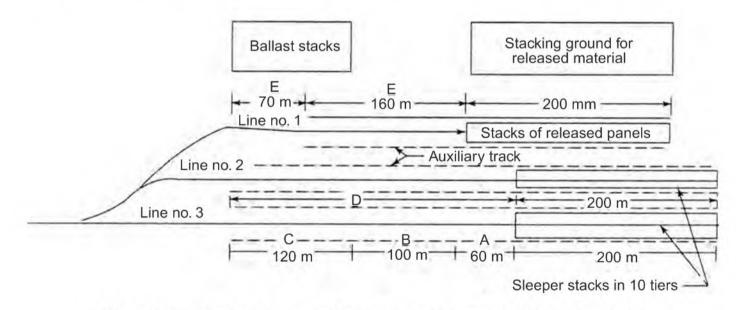
Fig. 15.5 Typical layout of a pre-assembly yard of relaying train
