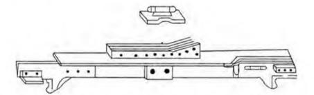
Fig. 14.4 Gauge-cum-level and spirit level
