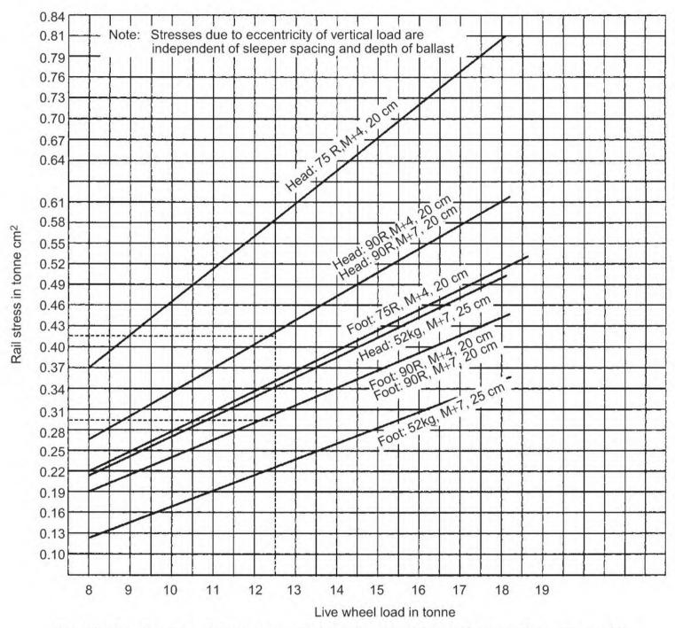
**Graph C** Stresses due to eccentricity of vertical load (for broad gauge track)
