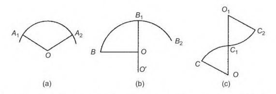
Fig. 6.2 Classification of curves: (a) Simple curve (b) Compound curve (c) Reverse curve
