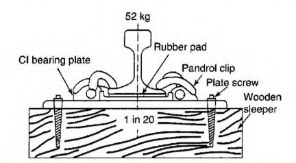
Fig. 5.26 (b) Pandrol clips with wooden sleepers and CI bearing plate
