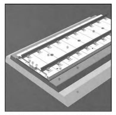
Fig. 18.3 Max Bogl slab track system (See also Color Plate 14)
