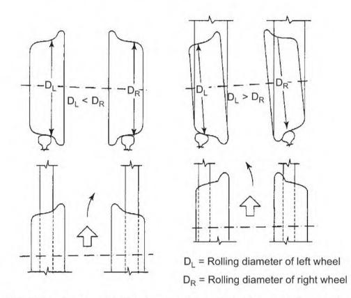
Fig. 22.19 Wheel set guidance by tread conicity through change in rolling dia
