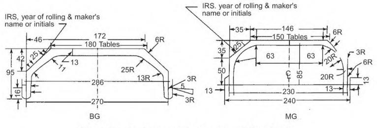
Fig. 4.12 Steel sleepers for turnouts—BG and MG
