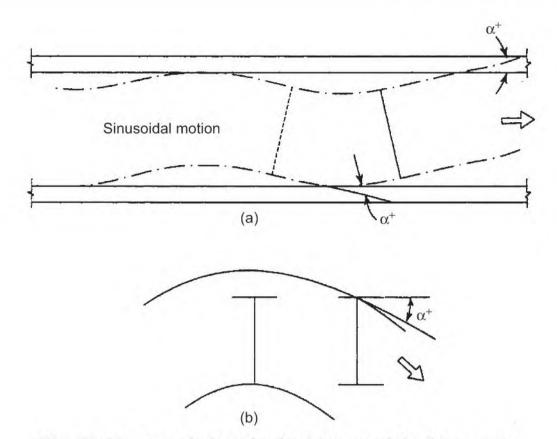
Fig. 22.15 Angularity of axle, (a) on straight (b) on curve
