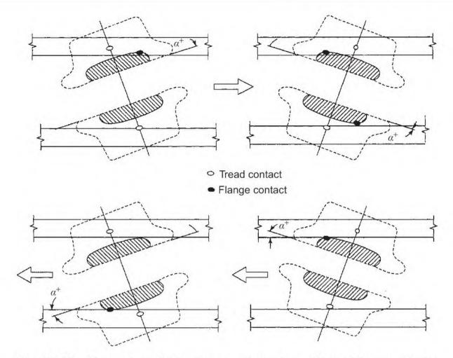
Fig. 22.12 Examples of wheel set configuration with positive angularity
