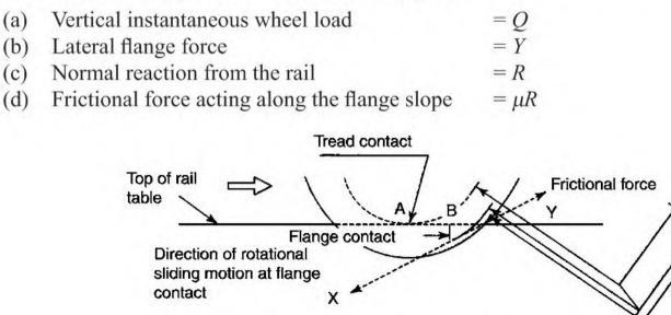
Fig. 22.10 Positive angularity (elevation)
