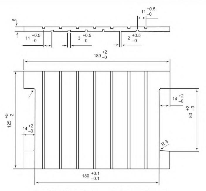
Fig. 5.23 6 mm thick grooved rubber pad with horns
