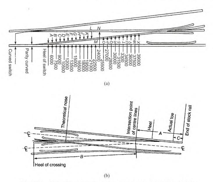
Fig. 7.17 Main dimensions for setting out turnouts (BG, MG and NG)
