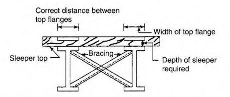
Fig. 21.1 (b) Making of notches for seating on girder flanges
