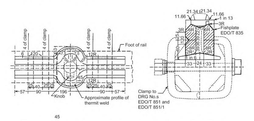
Fig. 10.14 Joggled fishplates with clamps for rail fractures BG for BS No. 90R
