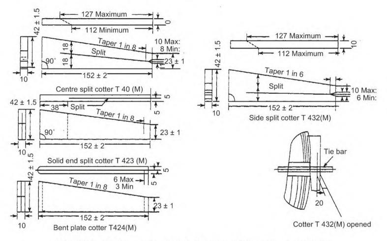
Fig. 5.21 CI sleeper fastening MS cotters (dimensions are in mm)
