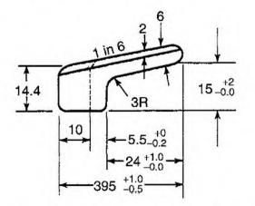
Fig. 5.30 Glass nylon insulating liner RDSO/T-2505
