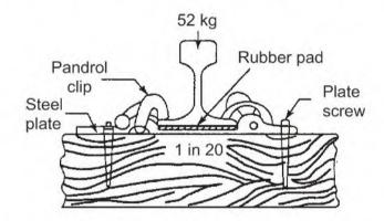
Fig. 5.26 (a) Pandrol clips with wooden sleeper and steel pad
