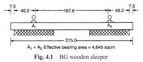
The standardized size of the wooden sleepers for use on various gauges in Indian Railways is given in Table 4.2.
