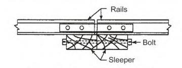
Fig. 3.5 (a) Supported joint
