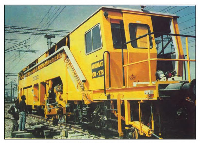
Fig. 12.11 (a) Points and crossing tamping machine
