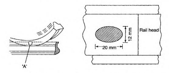
Fig. 19.6 Contact area between wheel and rail
