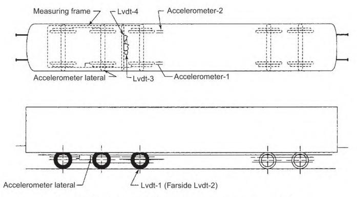
Fig. 17.12 Location of transducers in measuring vehicle
