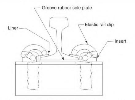
Fig. 5.29 Pandrol clips with concrete sleepers
