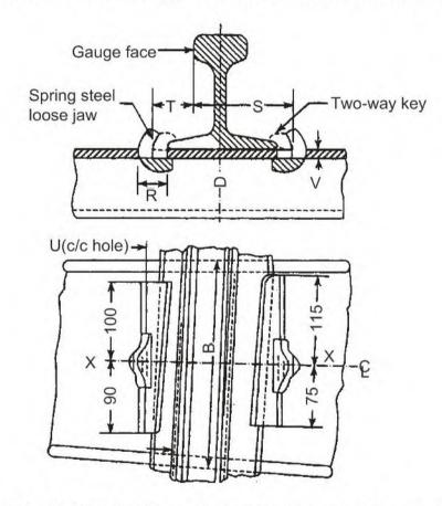
Fig. 5.17 BG and MG steel trough sleepers (plan at rail seat)
