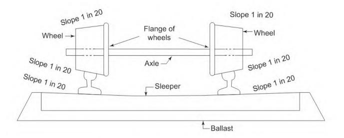
Fig. 1.5 Coning of wheels
