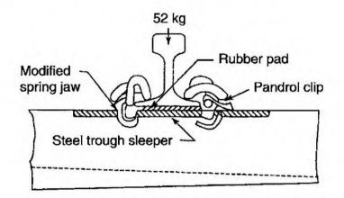
Fig. 5.28 Pandrol clips with modified spring jaws
