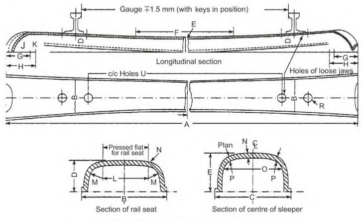
Fig. 4.11 BG and MG steel trough sleepers
