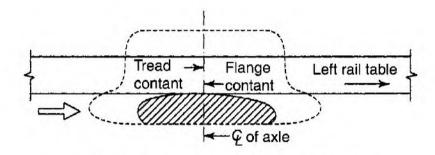
Fig. 22.7 Zero angularity (plan)
