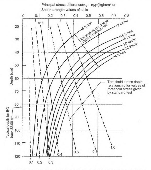
Fig. 8.4 Typical chart of induced stress and subgrade shear strength
