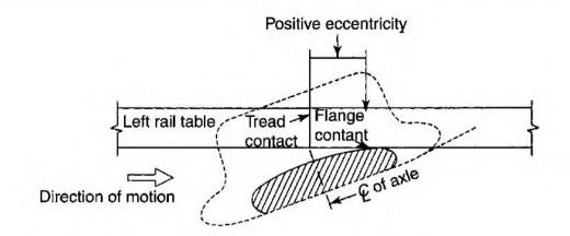
Fig. 22.8 Positive angularity (plan)
