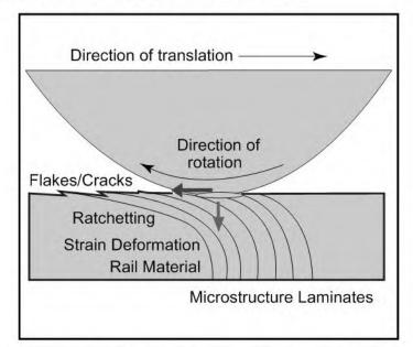
**Fig. 2.4** Contact patch pressure and forces causing surface elastic deformation of the rail microstructure, loading to RCF (See also Color Plate 1)
