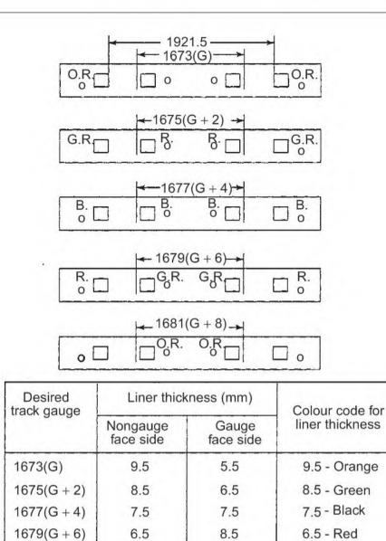
**Fig. 4.15** PSC sleeper for providing slack gauge on curves (identical sleepers different liners)
