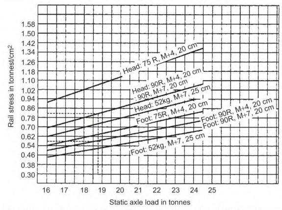
**Graph D** Stresses due to twisting effect under flange force (for broad gauge track)
