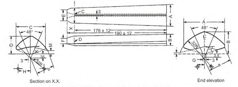
Fig. 5.13 Two-way keys (normal size)
