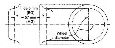
Fig. 22.35 Measurement of wheel tread diameter
