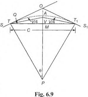
OT, TM and OM can be measured at site, and thus, the radius can be calculated.
