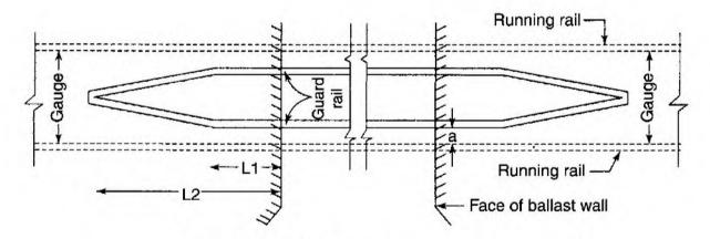
Fig. 21.2 A typical arrangement of a guard rail
