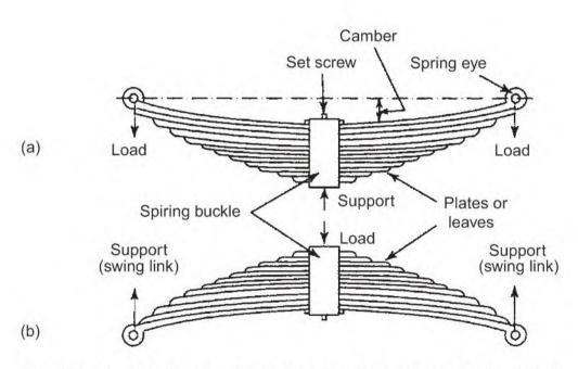
Fig. 22.41 Leaf or laminated spring (a) normal (b) inverted
