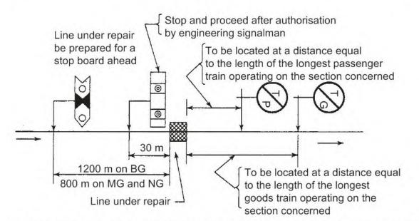
Fig. 11.6 Fixture of engineering indicators for dead stop restrictions outside station limits
