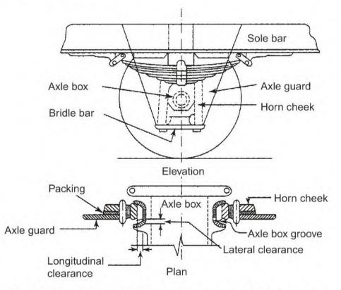
Fig. 22.40 Axle guard, horn cheek and axle box groove
