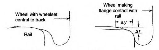
Fig. 22.22 Measurement of effective conicity
