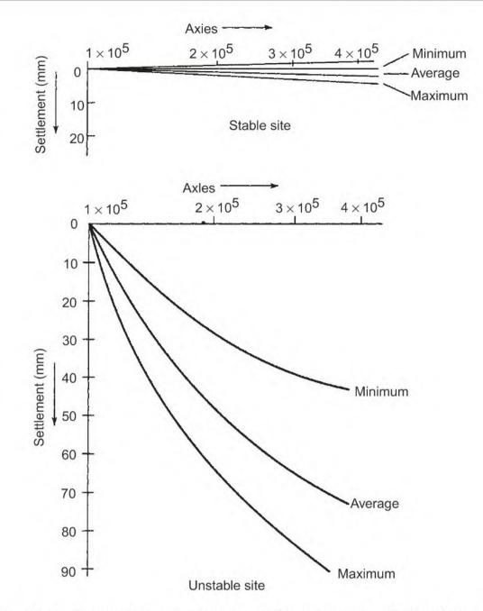
Fig. 8.7 Typical cumulative settlement of formation on stable and unstable sites
