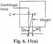
The resultant force XR acts toward the outer rail and thus exerts a greater load on the outer rail than the inner one. Further, if speed V is increased or radius, R is reduced, the centrifugal force will be greater, XC will be longer, while XW will remain the same and so XR will get nearer to the outer rail. When the conditions become such that the resultant passes through the outer rail; there is no load on the inner rail, and the vehicle is on the point of overturning.
