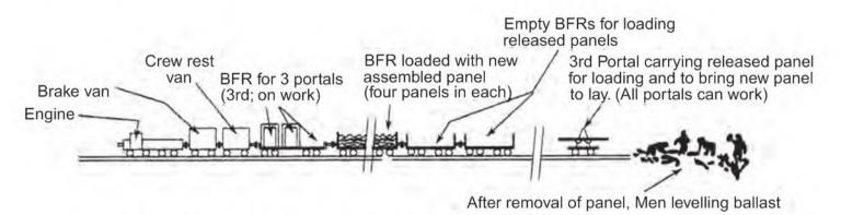
Fig. 15.6 A typical marshalling order of the relaying train for site working
