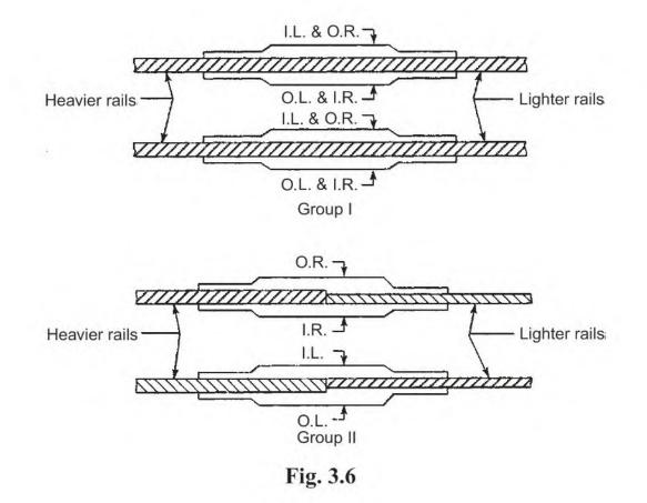
The IRS design of combination fishplates comprises two main groups or sections:
