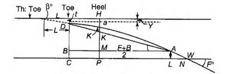
Fig. 7.16 IRS layout with curved switch
