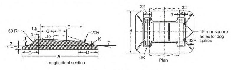
Bearing plate cast iron Fig. 5.7
