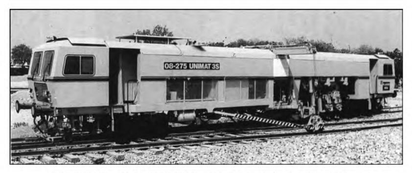
**Fig. 12.11 (b)** Unimat 08-275 3S switches and crossing tamping machine (See also Color Plate 5)
