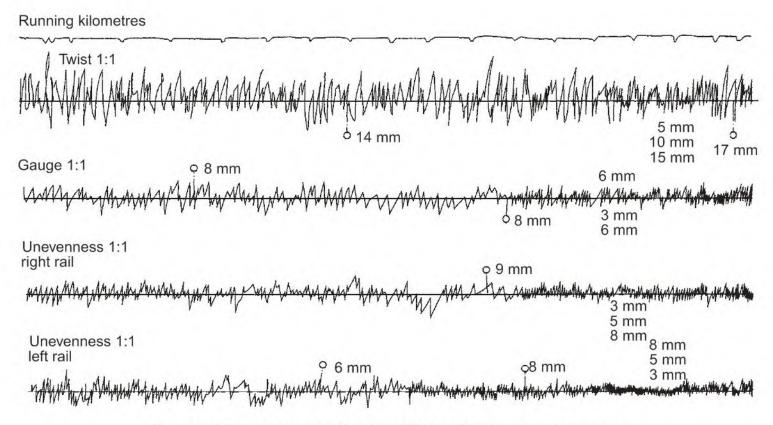
Fig. 17.2 (c) Sample chart of TRC (Electric) metre gauge
