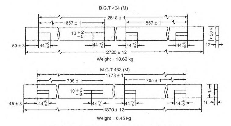
**Fig. 5.20** Cast iron sleeper fastenings (MS tie bars)
