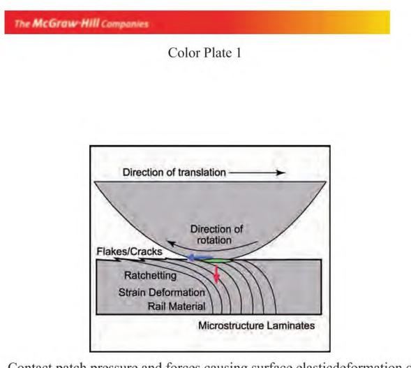
**Fig. 2.4** Contact patch pressure and forces causing surface elastic deformation of the rail microstructure, loading to RCF
