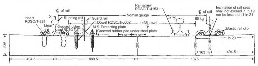
Fig. 4.17 Concrete sleepers for guard rails
