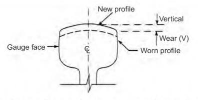
Fig. 15.1 A typical profile showing the measure of vertical wear of the rail
