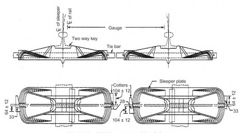
Fig. 4.10 CST-9 type assembly of sleeper
