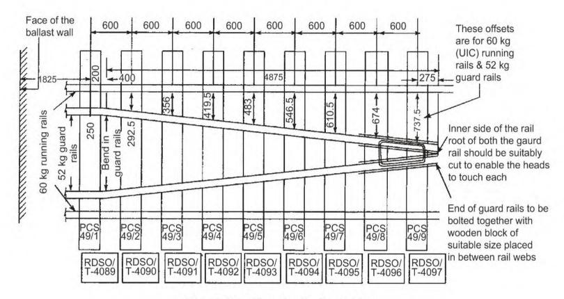
Fig. 5.41 Guard rails for bridges
