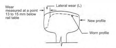
Fig. 15.2 A typical profile of the worn rail showing the measures of lateral wear
