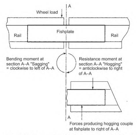
Fig. 3.1 Couple exerted on the fishing surfaces by wheel load
