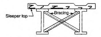
Fig. 21.1 (c) Notches cut in sleeper
