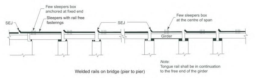
Fig. 10.6 Welded rails on bridge
