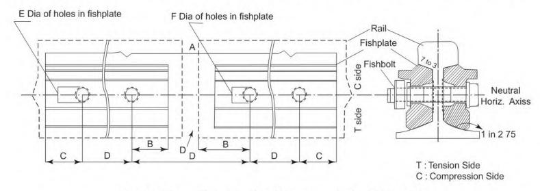
**Fig. 3.3 (c)** Fishplate for 52 kg rails (refer Table 3.3)
