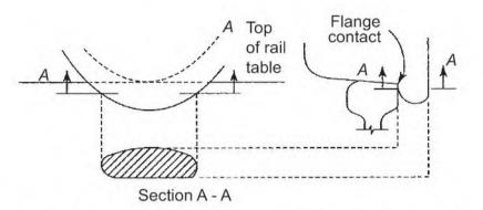
Fig. 22.6 Sectional plan of wheel flange at level of flange-to-rail contact
