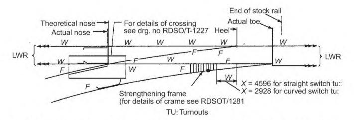
Fig. 7.29 LWR through points and crossings: W, welded joint; F, fishplated joint
