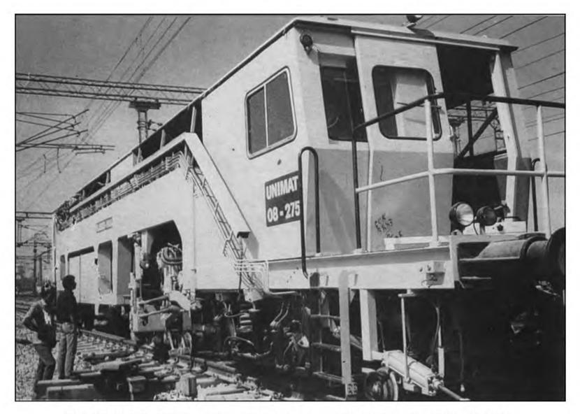
Fig. 12.11 (a) Points and crossing tamping machine (See also Color Plate 5)
