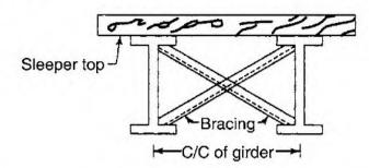
Fig. 21.1 (a) Preparation of bridge timber making rail seats in one plane
