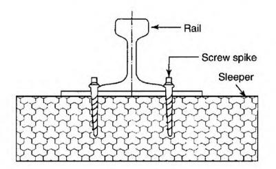
Fig. 5.4 Flat MS bearing plate
