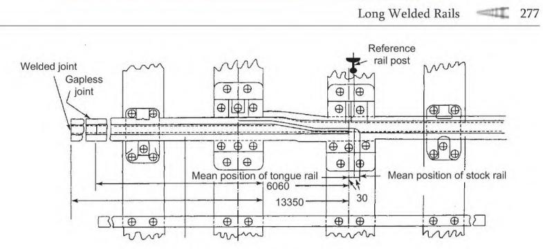
Fig. 10.3 Switch expansion joint
