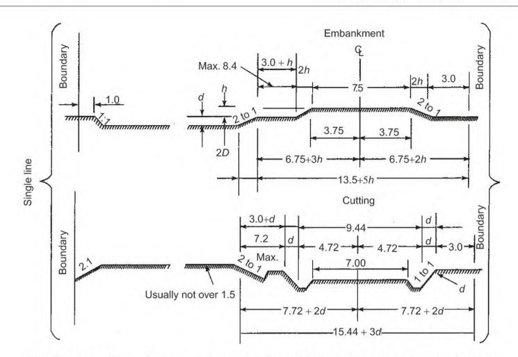
Fig. 8.6 (a) General cross-sections showing width of land to be taken up for BG
