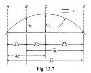
The track is measured at four points. The versine  $H_2$  at point *B* represents the measuring base. At point *C*, the lining slew is made till the vesine  $H_1$  is in correct ratio to  $H_2$  ( $H_1 = H_2 \times i$ ).
