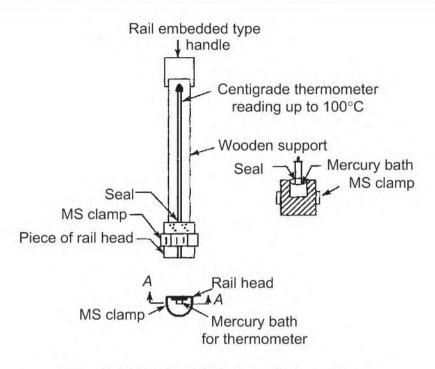
(a) Rail embedded type thermometer
