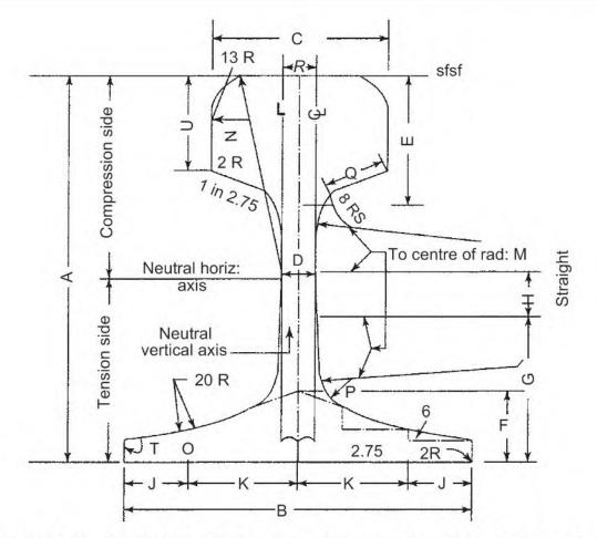
Fig. 2.3(a) I.R.S 52 kg F.F. rail section—key to table of dimensions
