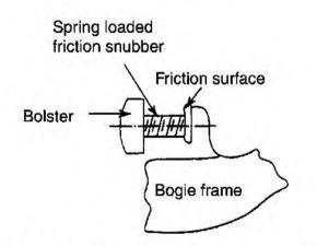
Fig. 22.44 Spring loaded friction snubber
