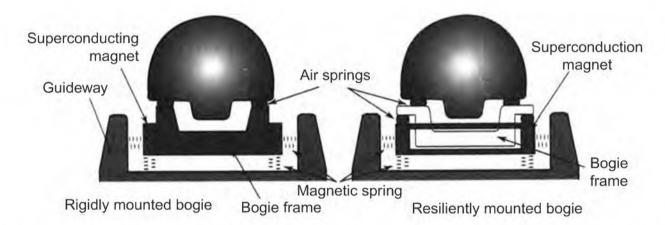
**Fig. 18.10** The second test train will have resiliently mounted bogie (right); the rigidly mounted bogie (left) is lifted on the first train
