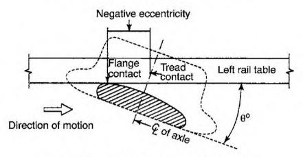
Fig. 22.9 Negative angularity (plan)
