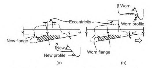
Fig. 22.16 Increase in eccentricity with increase in  $\beta$
