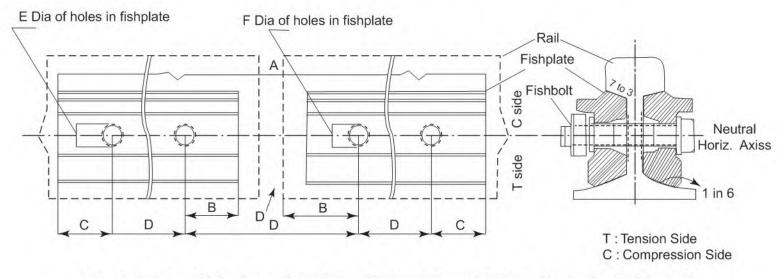
Fig. 3.3 (a) Fishplates for 50 R, 60 R, 75R and 90R rails (refer Table 3.1)
