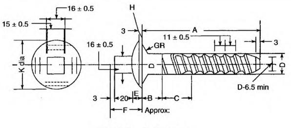
Fig. 5.3 Rail screws
