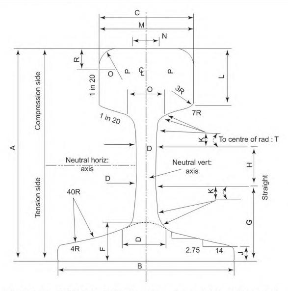
Fig. 2.3(c) UIC 60 kg F.F. rail section—key to table of dimensions
