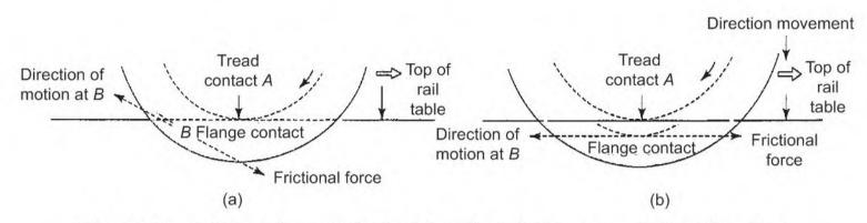
Fig. 22.11 (a) Negative angularity (elevation) (b) Zero angularity (elevation)
