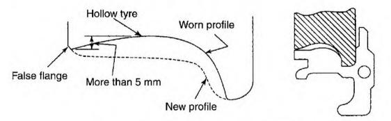
Fig. 22.34 False flange/hollow tyre
