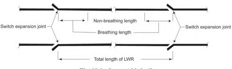
Fig. 10.1 Long welded rail
