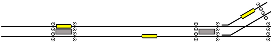
Figure 1. Fallback with secondary train detection at stations and junctions only
