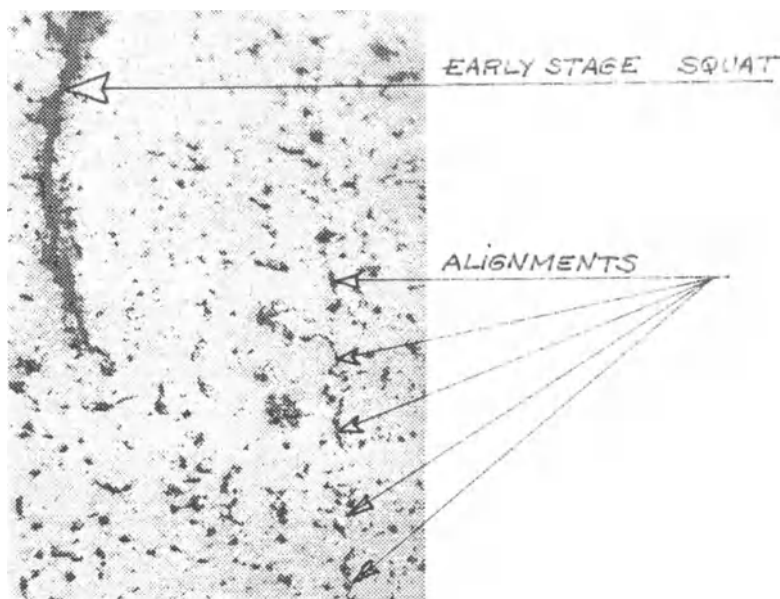
Fig. 11. Alignment of surface micro-cracks Optical microscope.
