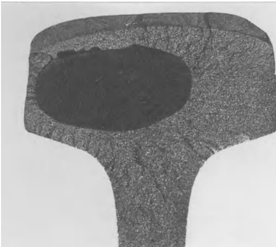
Fig. 1. An example of an incipient detail fracture of a rail in service. The rail is a Colorado Fuel & Iron 133 RE (AREA 133 lb./yd.) section, from Union Pacific Railroad track near Laramie, Wyoming, in service from 1957 to 1975. After detection of the internal crack, a section of rail containing the defect was removed from the track and broken at the AAR Chicago Test Center to reveal the fatigue crack submerged in the rail.
