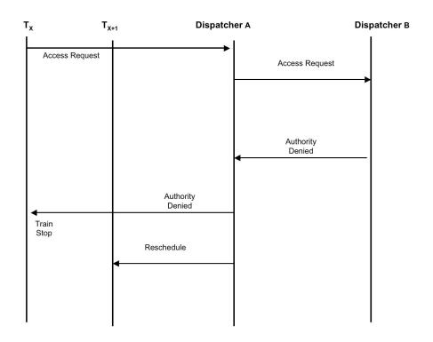
Figure 6.15: Lead Train Passes Security Check-Domain B Track Blocked
