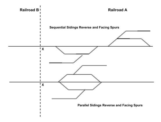
Figure 6.11: Sequential and Parallel Sidings with Facing and Reverse Spurs
