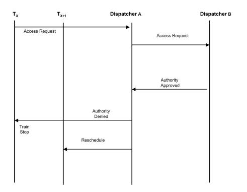
Figure 6.16: Lead Train Passes Security Check- Domain A Track Blocked
