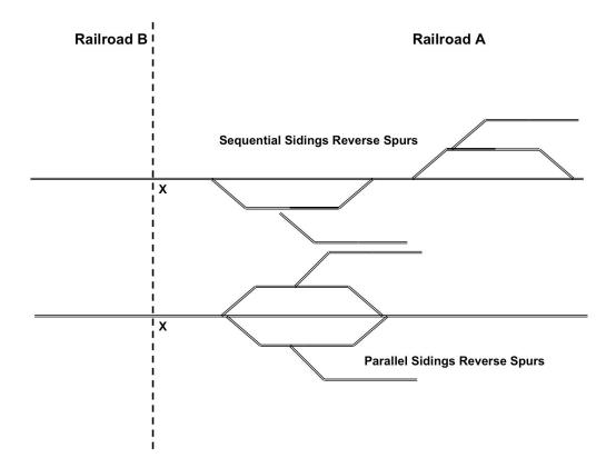
Figure 6.9: Sequential and Parallel Sidings and Reverse Spurs
