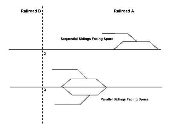
Figure 6.6: Sequential and Parallel Sidings and Facing Spurs
